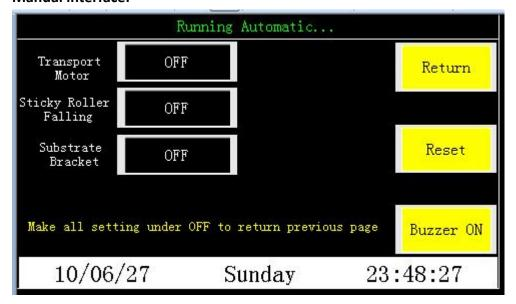
The motor can be transferred independently, cleaning operation, substrate holder on / off, if you want to return, be sure to put all the switches in the OFF position.
