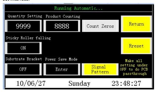
Open the "cleaning action" and "substrate support" PCB cleaning mode.
