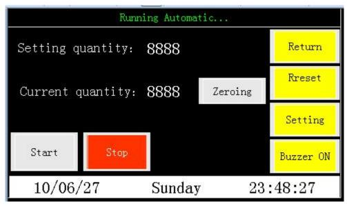
First enter the setup interface will need to set the function and click the "Start" button to enter the automatic production state.
